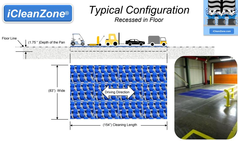
Effective solution for forklifts with tires = or < 14" Dia. wheels/roles + Walkthrough Configuration: 3 x 4 (12) iCleanZone-Std Grates Cleaning Area = (83" wide x 154 "Long) The optimum layout of the iCleanZone®, can vary depending upon the size and space available in each location.
