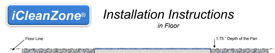
(1) Prep the installation area. The overall area to be 1" larger in width and length of the Cleaning Grate Area. The area to be recessed approximately 2" form the main surface of the floor (1.75" for the Pan height + 3/16" for the filler)
